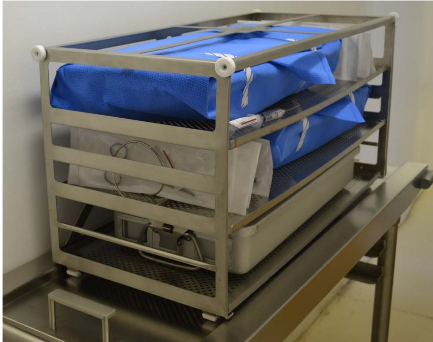
Figure 4. Validation load #3: three single channel flexible endoscopes with additional general medical devices
